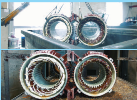
Double dip in class H varnish and double baking
