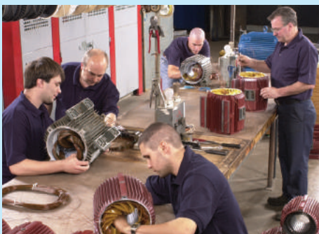
Handmade lap winding
