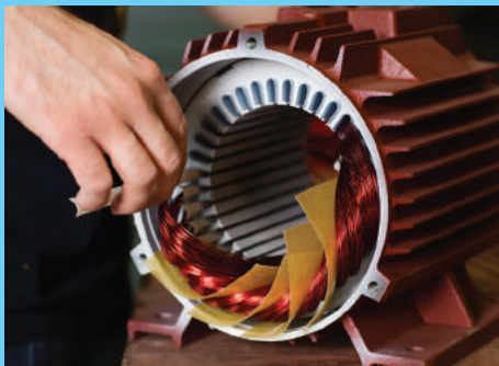
Phase to phase insulation
