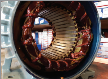
Less insulation between phases
