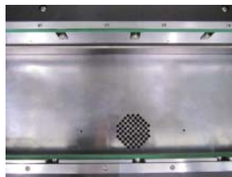
Vacuum absorption & Fan Blower for 0603mm and 0401mm chips.
